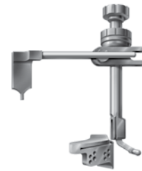
Figure 5 Locking Lever is in the “Closed” Position
