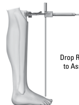
Figure 7 Use the Stylus to Reference the Tibial Plateau
