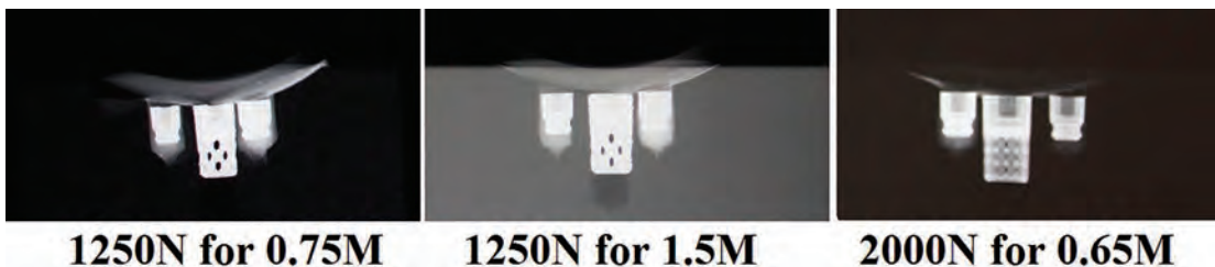
Figure 4 Representative radiographs of the new cage glenoid design after superior glenoid rim edge loading for 1,250 N for 0.75 M cycles in a low density block (left), 1,250 N for 1.5 M cycles in a high density block (middle), and 2,000 N for 0.65 M cycles in a high density block (right).
