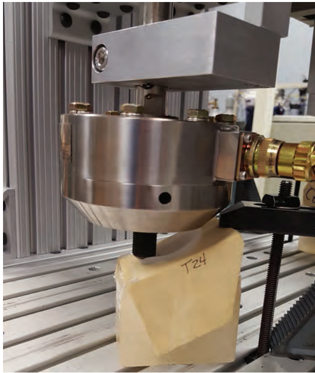
Figure 2 Representative image depicting cyclic loading along the superior glenoid rim when loaded at 2000 N. Superior glenoid rim plastic deformation is evident at these elevated loads.
