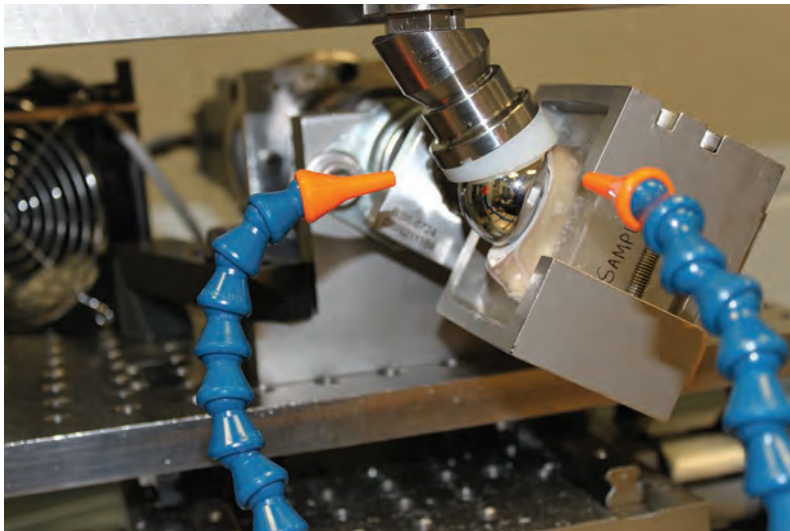
Figure 3 Representative image of the rTSA glenoid loosening cyclic test.
