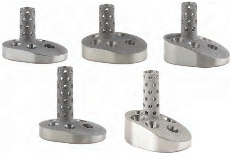
Figure 1 Equinox® baseplates (Exactech, Inc., Gainesville, FL). Top row from left to right: standard baseplate, 8° posterior augment, 10° superior augment; bottom row from left to right: +10 mm extended cage and 10° superior/8° posterior augment baseplate.
